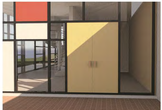
picture No.14 3d View // placing doors in curtain walls
