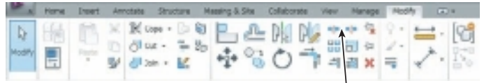
Figure 3.88 Locating the Split tool on the Modify tab to split a wall
