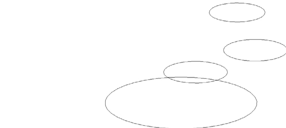
Figure 7.21 Bad loft cross section shapes
