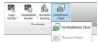
Figure 19.8 Interference Check button
