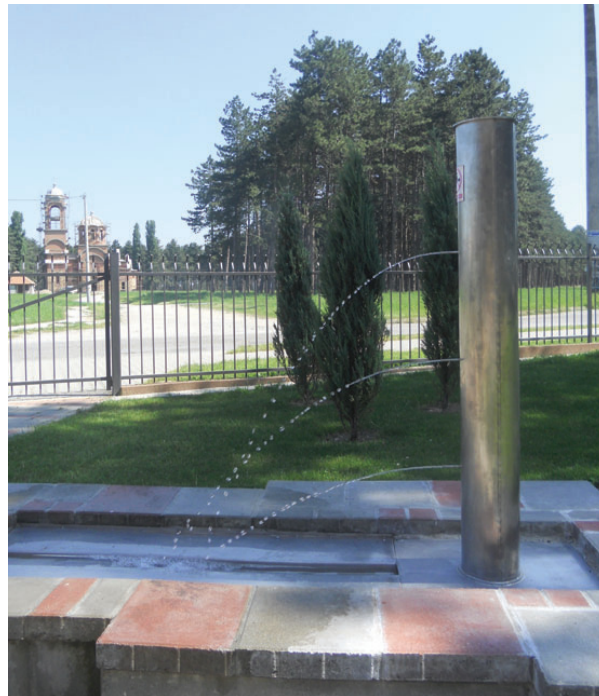
Fig. 1. Torricelli's fountain 13 located in the Center for Advancement of Educators in Šabac, Serbia, exemplifies well the parabolic jet pattern found by Torricelli.
