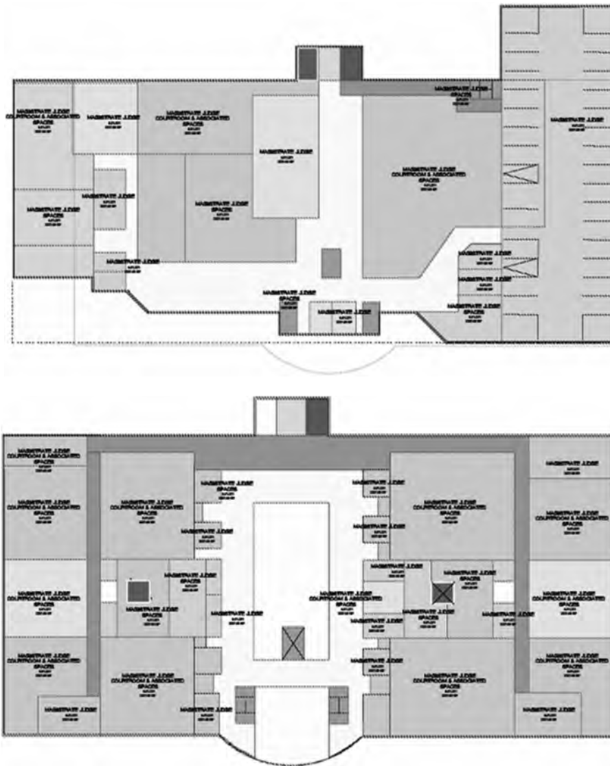
FIGURE 5-7 Example BIM model of a preliminary concept design for a two-story courthouse.
