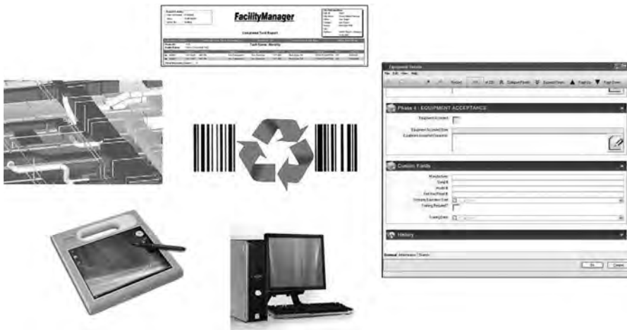
FIGURE 9-4-4 BIM and facilities management integration. Input of model and field data to the Tekla model and the CMMS using barcode identities.
