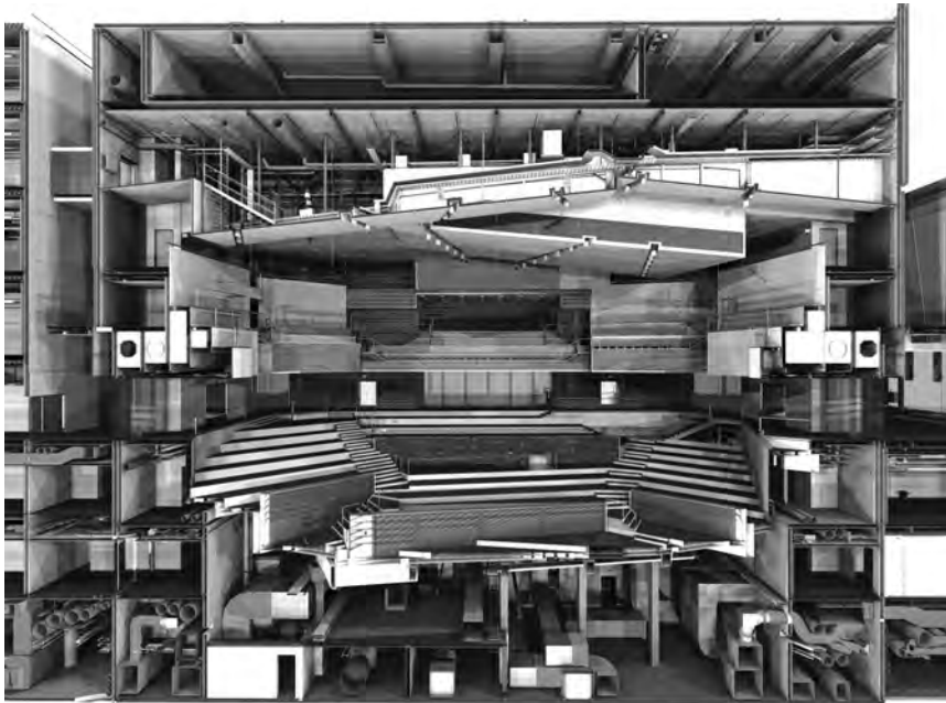
FIGURE 9-8-13 Combined model for layout and clash detection.
